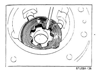
4. Arrange the friction discs so that the splines of the side gear can be inserted.
