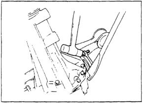
9. Tap the output shaft with a plastic hammer as shown in the figure to remove the output shaft.
