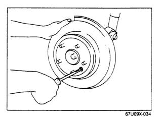
6. Remove the set screws and disc plate.
