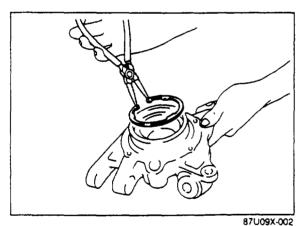
11. Remove the retaining ring from the toe control hub using snap ring pliers.
