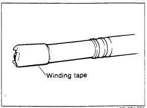
7. Wrap the spline of the shaft with tape to prevent damaging the boot, remove the boot.
