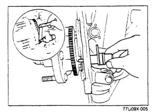
8. Install the speed sensor, and check the clearance between the sensor rotor and speed sensor.
