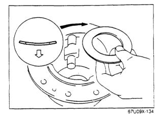
2. Install the conical springs.
