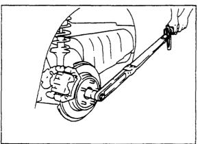
Tighten the lock nut.
