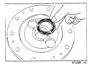
11. Coat the thrust washer with grease and install it in the differential cover.
