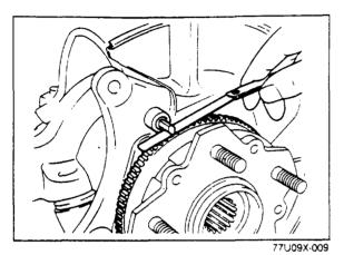
2. Install the speed sensor, and check the clearance between the speed sensor and sensor rotor.
