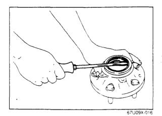
3. Remove the oil seal and the bearing.
