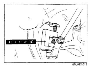
7. After removing the cotter pin and tie-rod end nut, use **ball joint puller** (49 0118 850C) to separate the tie-rod end from the knuckle.
