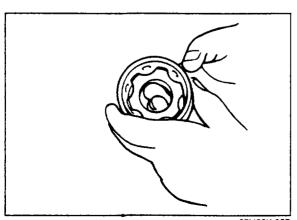
6. Turn the cage about 30°, and separate it from the inner ring.
