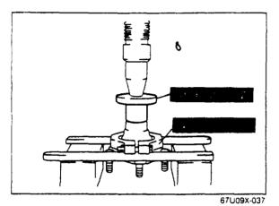
10. Press the wheel hub using **bearing installer** (49 F026 102) and **fan pulley boss puller** (49 0636 145) and remove the wheel bearing inner race.
