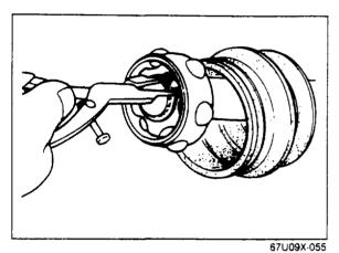
3. Remove the snap ring using snap ring pliers.
