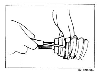
Fold the band back over itself while pulling on the end of the clip with pliers.
