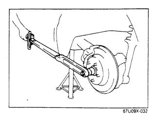
4. Depress the brake pedal to hold the hub secure, and then remove the hub nut.
