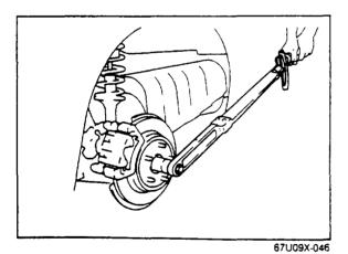
3. Depress the brake pedal to secure the disc plate, and tighten the lock nut.
