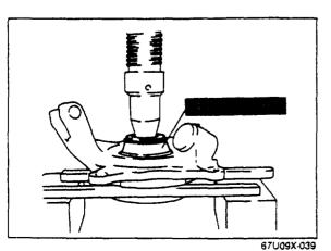
12. Remove the wheel bearing outer race using attachment (49 F027 007).
