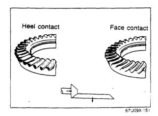
(2) Heel and face contact Replace the spacer with a thicker one, and bring the drive pinion closer in.
