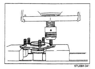
4. Check the wheel lug bolts for wear or damage. Replace the wheel lug bolts using a press, if necessary.
