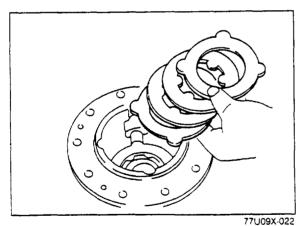
3. Install the friction plates and disc.
