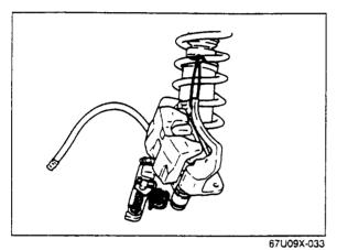
5. Remove the caliper assembly and suspend it using a rope.
