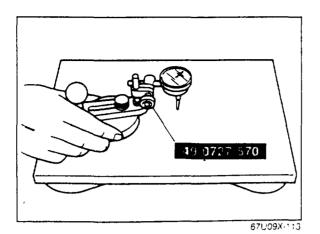
7. Place the **pinion height adjust gauge body** (49 0727 570) on the surface plate and set the dial indicator to "Zero".
