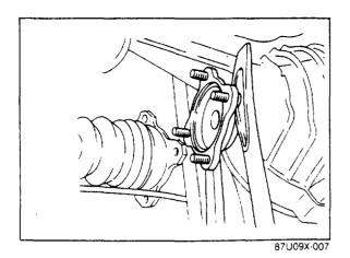
2. Insert two pry bars between the differential case and the output shaft, remove the output shaft by applying pressure to the pry bars.
