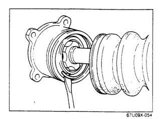
2. Remove the clip with a screwdriver.
