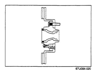
5. Apply grease (lithium base, NLGI NO. 2) to the shaded areas as shown in the figure.
