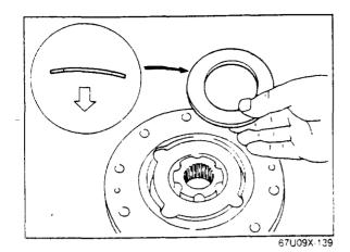
10. Install the conical springs.
