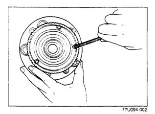
4. Remove the sensor rotor using a hexagon wrench.
