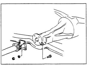
4. Install the propeller shaft.
